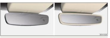
Fig. 62 Rear-view mirrors with automatic dimming: variant 1/2
