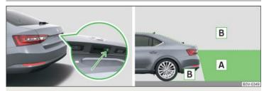
Fig. 174 Installation location of the camera / scanned area behind the vehicle
