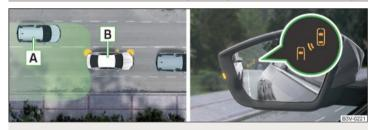
Fig. 172 Driving situation / indicator light in the left outside mirror indicates the driving situation
