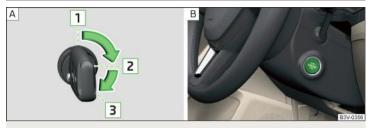
Fig. 150 Positions of the vehicle key in the ignition lock / starter button
