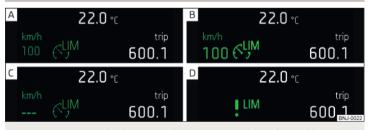
Fig. 189 MAXI DOT display (monochromatic): Examples of speed limiter status displays
