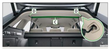
Fig. 140 Correctly secure net partition behind the front seats in the pulled-out state
