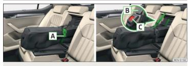
Fig. 101 Tighten ribbon / secure through-loading bag
