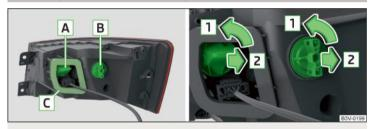
Fig. 266 Tail light / bulb replacement
