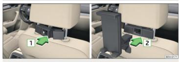
Fig. 111 Inserting: adapter / holder
