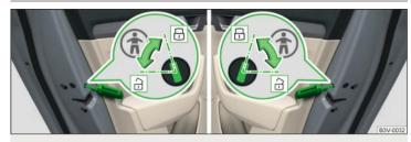
Fig. 35 Switching on/off the parental control: rear door left/right
