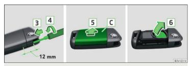
Fig. 243 Replacing the battery
