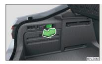
Fig. 71 Fold the backrest forward from the luggage compartment
