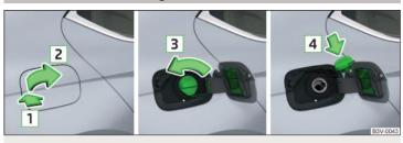
Fig. 213 Open fuel filler flap / unscrew tank cap / place the tank cap on the fuel filler flap
