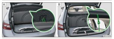
Fig. 120 Fastening the flooring: variant 1/2
