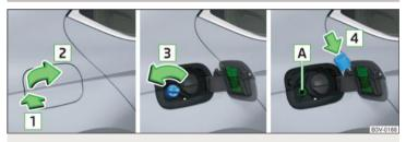
Fig. 215 Open fuel filler flap / unscrew tank cap / place the tank cap on the fuel filler flap
