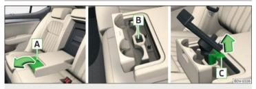
Fig. 113 Open storage compartment / stowage compartment for holder / remove holder
