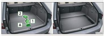
Fig. 137 Fold up variable loading floor / folded variable cargo floor in the upper position
