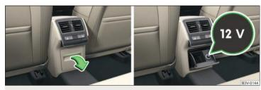
Fig. 106 Open storage compartment / cover of the 12 volt power outlet
