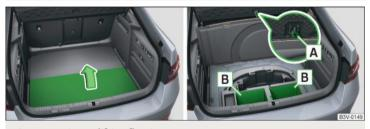
Fig. 131 Variant 1: lifting flooring & storage compartments
