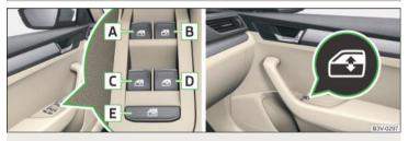
Fig. 40 Window lifter buttons
