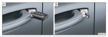
Fig. 247 Handle on the driver's door: key with fold-out key bit / KESSY emergency key
