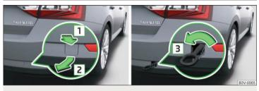
Fig. 240 Remove cap / install towing eye
