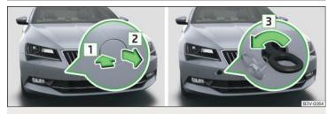
Fig. 239 Remove cap / install towing eye
