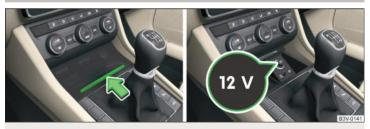
Fig. 104 Open storage compartment / cover of the 12 volt power outlet
