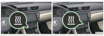
Fig. 148 Button for switching on / off the Climatronic / manual air conditioning
