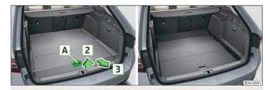
Fig.  $136\,$  Set variable loading floor to the lower position / variable loading floor in the lower position
