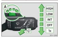
Fig. 59 Operating the windscreen wipers and washing system at the front
