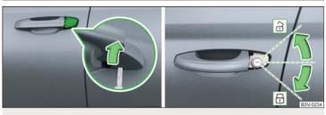
Fig. 246 Handle on the driver's door: unfold/lock and unlock the lock cover
