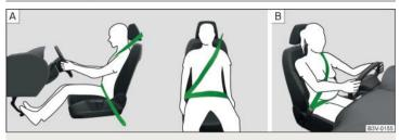
Fig. 4 Routing of belt webbing over the shoulders and the lap belt/Routing of belt webbing for an expectant mother
