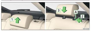
Fig. 74 Setting the height of the rear headrest
