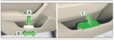
Fig. 87 Waste container: inserting and moving / opening
