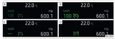
Fig. 186 MAXI DOT display (monochromatic): Examples of CCS status displays
