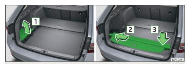
Fig. 125 Remove the left side cover / store roll-up cover
