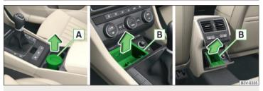
Fig. 109 Remove front ashtray / remove front ashtray insert / remove rear ashtray insert
