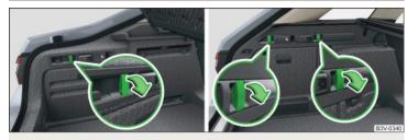
Fig. 119 Fold down hooks: variant 1/2
